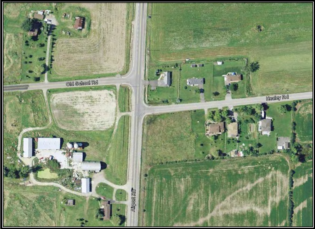
Figure 3: Offset intersections of Healey Road and Old School Road (Source: Google Earth)
