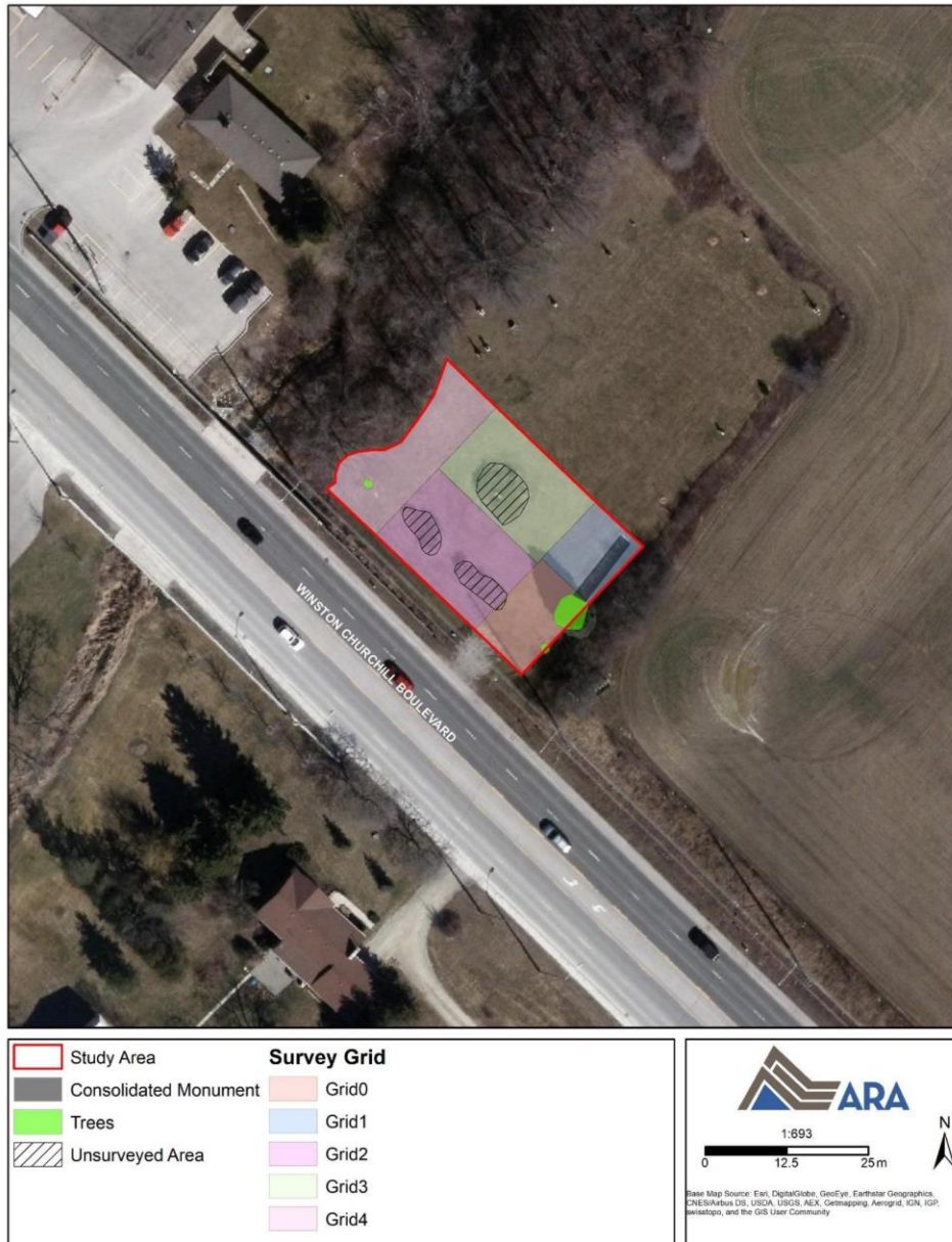
Figure 3: GPR collection grids.
