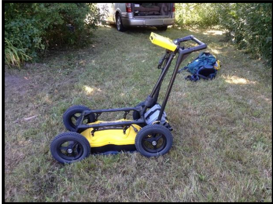
Image 11: GPR Survey Instrument (Stock Photo)
