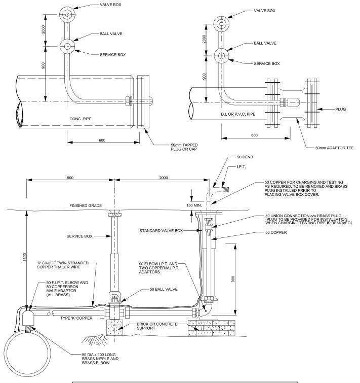
BLOW-OFF SIZE TO MATCH THE SIZE OF THE FEED BASED ON STANDARD DRAWINGS 1-7-7 AND 1-7-8. WHERE A 100mm FEED IS REQUIRED CONTRACTOR TO PROVIDE AN INSTALLATION, INCLUDING ALL NECESSARY MATERIALS, TO RESPECT THE DESIGN CONCEPTS OF THIS STANDARD DRAWING.
