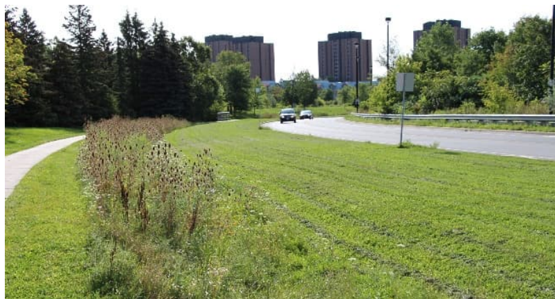
Figure 6.10 – SWM Alternative 9 Enhanced Ditches
