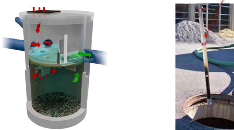
Figure 6.7 – SWM Alternative 6 Oil and Grit Separators
