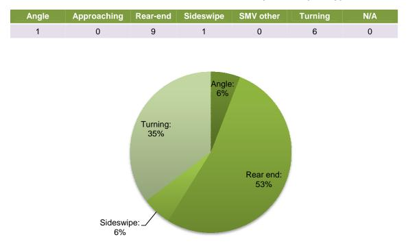
The collision frequency (3.4 per year) and collision rate (0.28 collisions per million intersecting vehicles) are among the lowest of signalized intersections within the Cawthra Road corridor, with a typical pattern of collisions observed.
