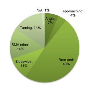
There was also a relatively high prevalence of single motor vehicle (SMV) collisions caused by loss of control on the eastbound and westbound approaches to this intersection. Much like the North Service Road, these approaches have sharp bends as illustrated in the collision diagram in **Appendix A**. Given that almost all of the loss-of-control collisions at this intersection occurred in wet, snowy or otherwise inclement weather conditions, it should be investigated how the
