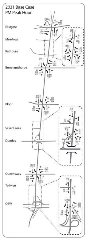
The **Eastgate Parkway** intersection is expected operate at LOS F during the AM and PM peak hours. Several movements will operate at LOS D or above due to opposing flows in all directions. The northbound left turn had the highest frequency of left turn collisions.
