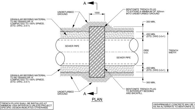
UNSHRINKABLE CONCRETE MAY BE USED AS AN ALTERNATE TO BENTONITE CLAY PLUG
