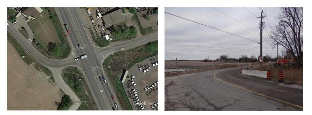
Figure 3: Skewed Intersection (Colerain Drive and Region Road 50)
