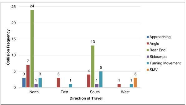
Figure 3: Collision Impact Type (Coleraine Drive and Regional Road 50)
